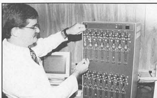
Test tubes — Jay Officer uses a purge trap tool to catch volatile hydrogens for analysis in the new environmental lab.
