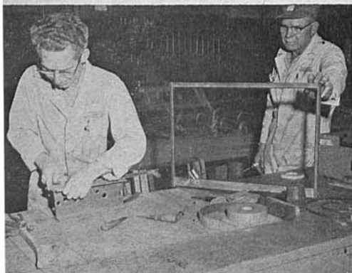
PREVENTING RATTLES in windows and doors keeps riders happier. Clarence Beard replaces felt in side runner of window. Sash is being held by Al Pyles.
