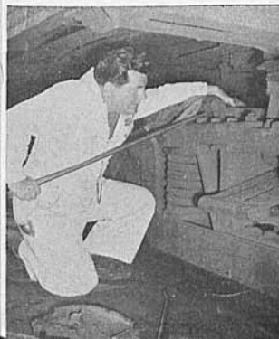
RAIL MAINTENANCE LEADERS —Photo at left: Paul R. Cloutier, second shift leader, replaces brake shoe on interurban car. Center photo: Frank E. Hadsell, third shift leader, left, inspects adjustment by Mechanic Thomas Cassidy of group switches underneath rail car. Photo at right: Mathew Laakson, first shift leader, adjusts relay that controls speeds of car.
