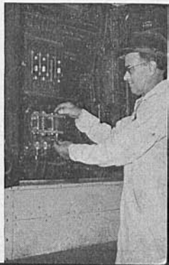
RAIL MAINTENANCE LEADERS —Photo at left: Paul R. Cloutier, second shift leader, replaces brake shoe on interurban car. Center photo: Frank E. Hadsell, third shift leader, left, inspects adjustment by Mechanic Thomas Cassidy of group switches underneath rail car. Photo at right: Mathew Laakson, first shift leader, adjusts relay that controls speeds of car.
