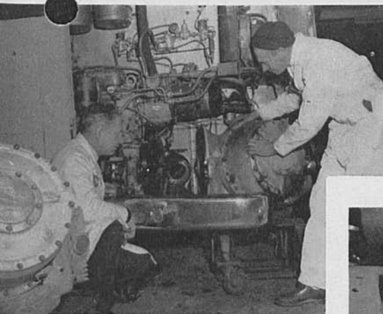
TURBINE , or fluid drive transmission, being removed at Ocean Park for mileage inspection at South Park Shops. Replacement turbine is in foreground. Night Foreman Earl Zwiebel, left, inspects the work of Mechanic Wm. R. Stosberg.
