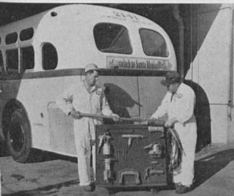
TURBINE , or fluid drive transmission, being removed at Ocean Park for mileage inspection at South Park Shops. Replacement turbine is in foreground. Night Foreman Earl Zwiebel, left, inspects the work of Mechanic Wm. R. Stosberg.
