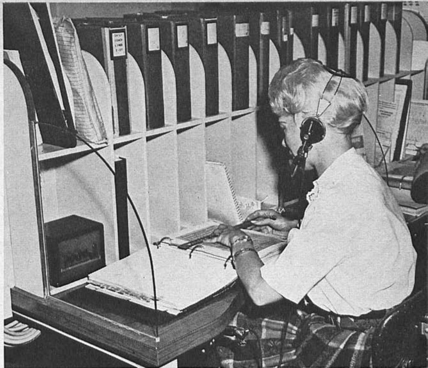
NEW-STYLE information station. Loretta Klitgaard is the Operator. Note small box with but two signal lights in pigeonhole at left. Green light means she is working on a call; amber light comes on to indicate that a call is waiting. She is not aware of the total number of calls waiting, as in the old-style set-up. Nervous tension is thus reduced. Note also the curved glass plates separating stations in order to reduce distraction that might be caused by the next Operator's voice, and to create more privacy.
