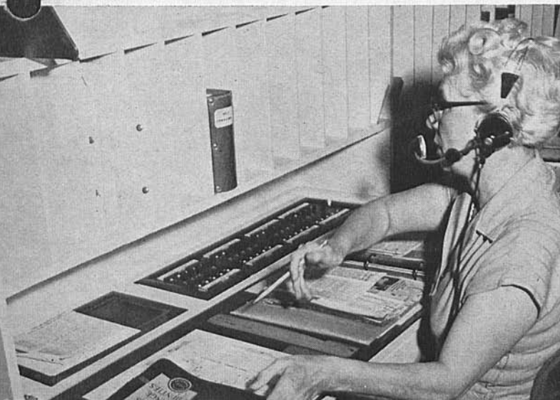
OLD-STYLE station at the information board. Isabel Ash is the Information Operator. Note the large number of signal lights on the switchboard. Operator could tell by number of glowing red lights number of waiting calls.
