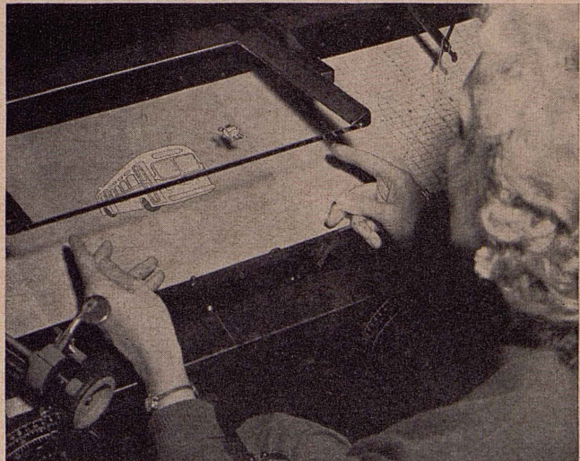
ARRANGING CELLS into a frame to be filmed. One sheet of transparent plastic is one cell. Frame consists of one to six cells.
