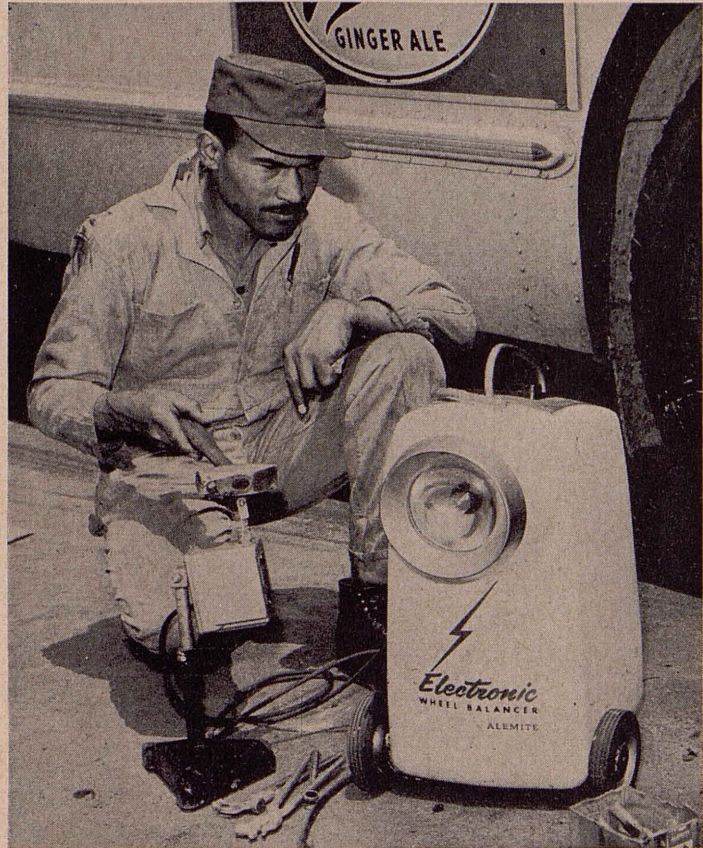
LONNIE MARKS , Macy mechanic, demonstrates the electronic wheel balancer now in use at Macy. The little box on a stand at left has a strongly magnetized arm which is placed in contact with the axle or brake backing plate to detect vibration. Lonnie holds a hammer head out to show how arm is magnetically attracted. Vibrations caused by unbalanced wheel are transmitted electrically to the stroboscope (machine on wheels), which has an intermittently flashing light by means of which the location of the unbalance is determined. A dial on the stroboscope shows the exact amount of counterbalancing weight needed.
