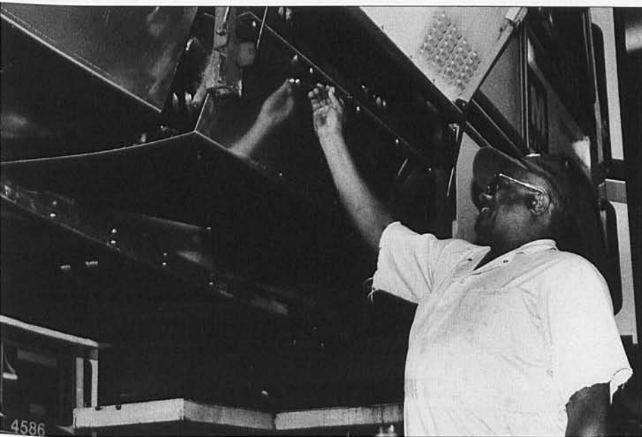
Division 8 mechanic Alex Rocio inspects the protective shields on the underside of a CNG bus.
