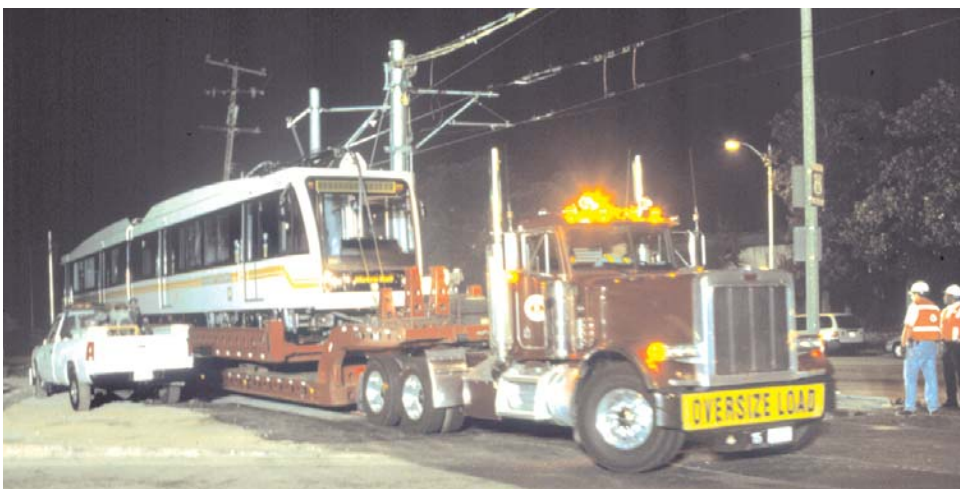
The first of six Metro Gold Line test cars is delivered alongside tracks in South Pasadena on a big-rig truck with an oversized trailer. Each car weighs 49 tons and is 89 feet long.
