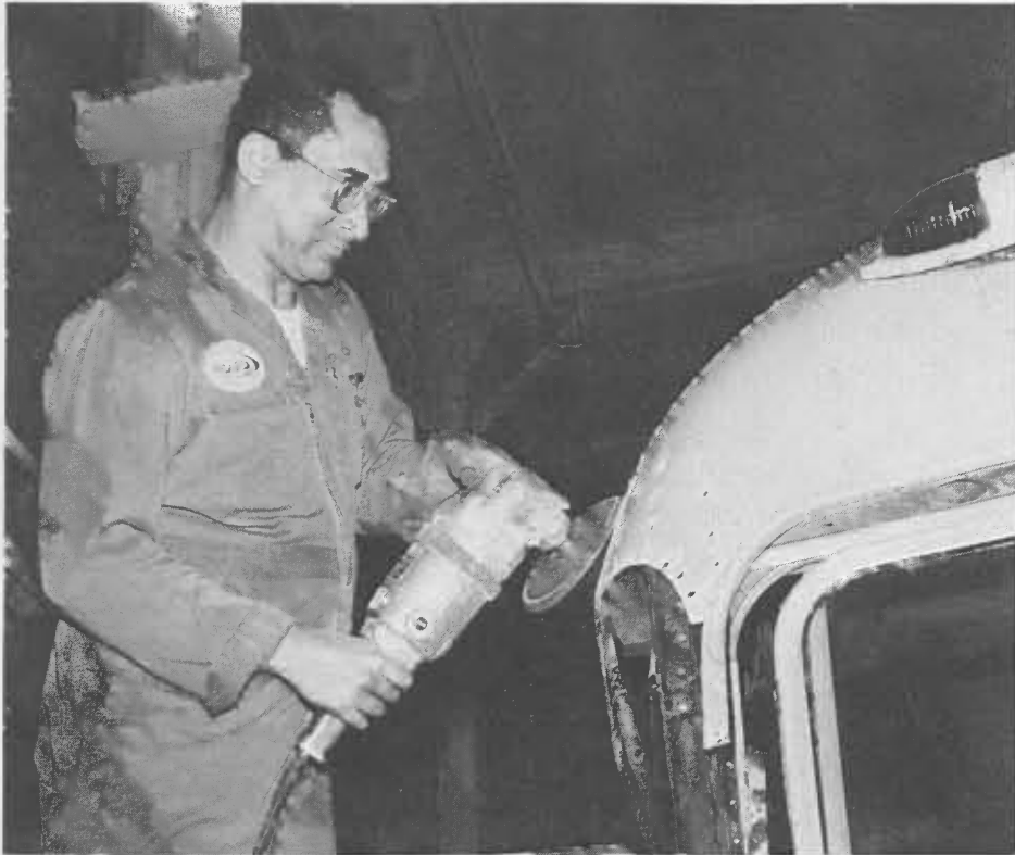
Horton Thomas, mechanic "B", uses a disc-sander in an accident repair task. Thomas has been with RTD since June, 1971.
