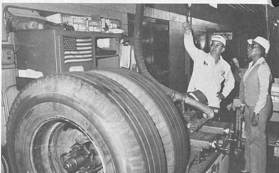
ROUND AND ROUND SHE GOES —Ted Hustava explains operation of a brake lathe to Jacquie Smith during a safety inspection at the Division 9 maintenance facility.
