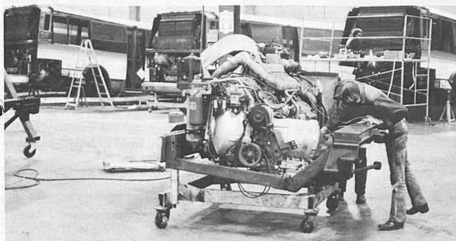
In the massive Carson facility (top) Grumman workmen labor over District GFC 870s to get them back on the streets. It takes a lot of manpower to perform the retrofit program, because virtually the entire undercarriage is removed in addition to the engine (below, left). Axle assembly is being removed from the old A-frame (at rear, below, right) while modified A-frame (foreground) is prepared for installation. At the bottom of the page is a diagram of the 870 undercarriage pinpointing the parts targeted in the retrofit program, and photo above that shows the four structural assemblies with new steel painted white. (Photos courtesy Bus World Magazine).
