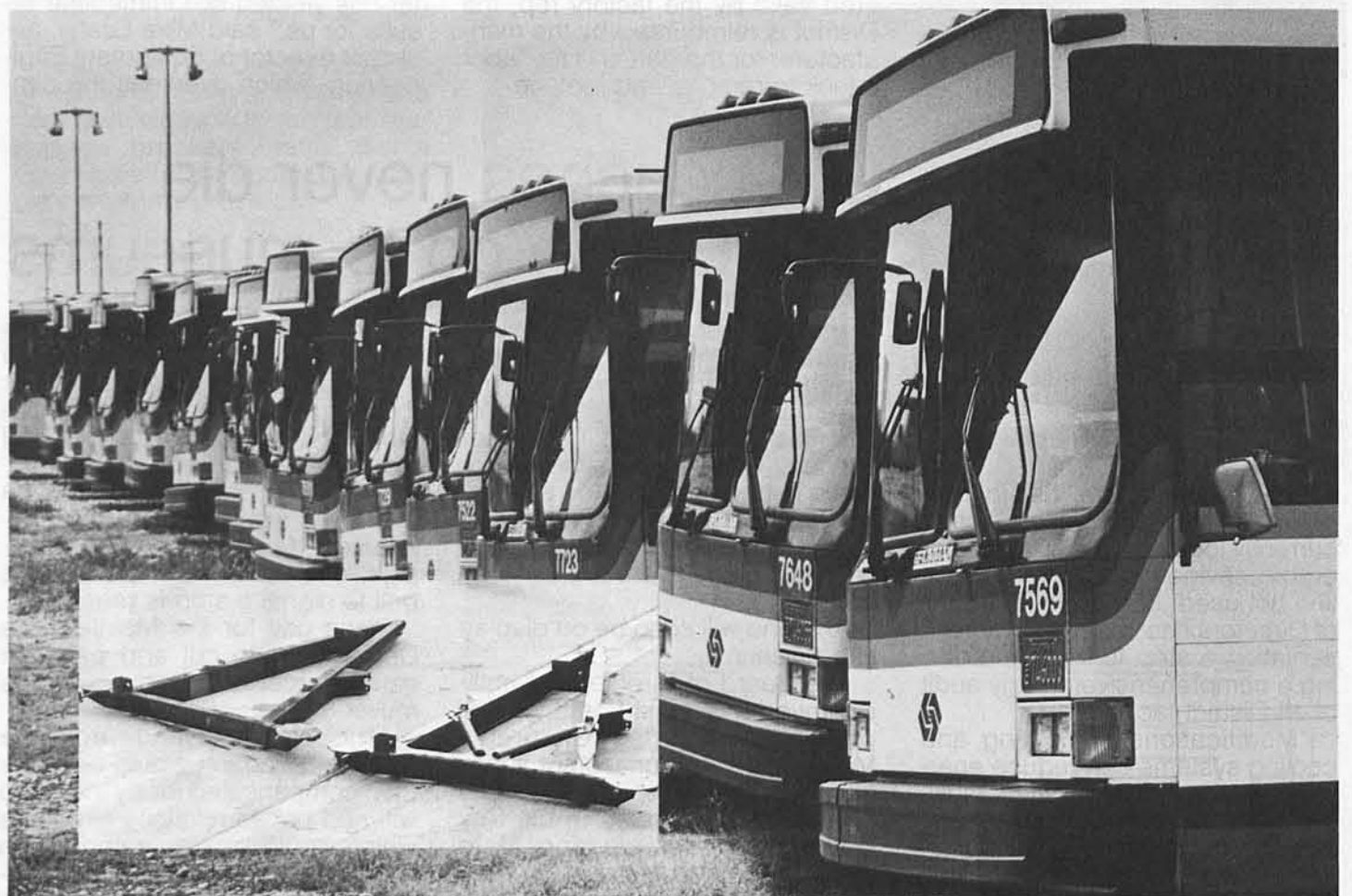
ON THE ROAD AGAIN — Grummans in storage awaiting repair, and (inset) the infamous A-frame before (left) and after (right).
