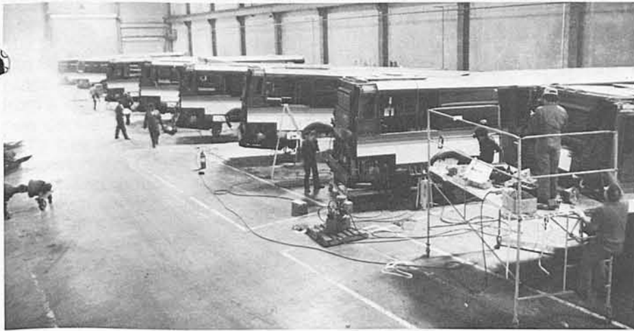
In the massive Carson facility (top) Grumman workmen labor over District GFC 870s to get them back on the streets. It takes a lot of manpower to perform the retrofit program, because virtually the entire undercarriage is removed in addition to the engine (below, left). Axle assembly is being removed from the old A-frame (at rear, below, right) while modified A-frame (foreground) is prepared for installation. At the bottom of the page is a diagram of the 870 undercarriage pinpointing the parts targeted in the retrofit program, and photo above that shows the four structural assemblies with new steel painted white. (Photos courtesy Bus World Magazine).
