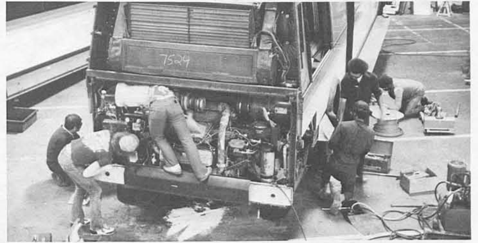
In the massive Carson facility (top) Grumman workmen labor over District GFC 870s to get them back on the streets. It takes a lot of manpower to perform the retrofit program, because virtually the entire undercarriage is removed in addition to the engine (below, left). Axle assembly is being removed from the old A-frame (at rear, below, right) while modified A-frame (foreground) is prepared for installation. At the bottom of the page is a diagram of the 870 undercarriage pinpointing the parts targeted in the retrofit program, and photo above that shows the four structural assemblies with new steel painted white. (Photos courtesy Bus World Magazine).
