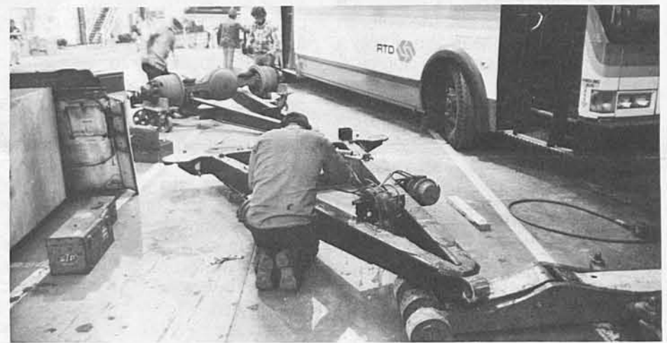
In the massive Carson facility (top) Grumman workmen labor over District GFC 870s to get them back on the streets. It takes a lot of manpower to perform the retrofit program, because virtually the entire undercarriage is removed in addition to the engine (below, left). Axle assembly is being removed from the old A-frame (at rear, below, right) while modified A-frame (foreground) is prepared for installation. At the bottom of the page is a diagram of the 870 undercarriage pinpointing the parts targeted in the retrofit program, and photo above that shows the four structural assemblies with new steel painted white. (Photos courtesy Bus World Magazine).
