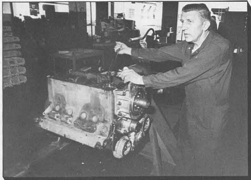
5 Next the engine moves to where Ray Krill inserts the pistons, connecting rods and oil pump.
