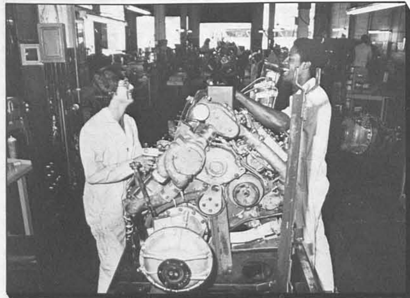
9 At the next station, Curtis Clark (left) and Wilfred Young team up to install the engine cradle, valve covers, transmission (which has been rebuilt), starter and oil cooler.
