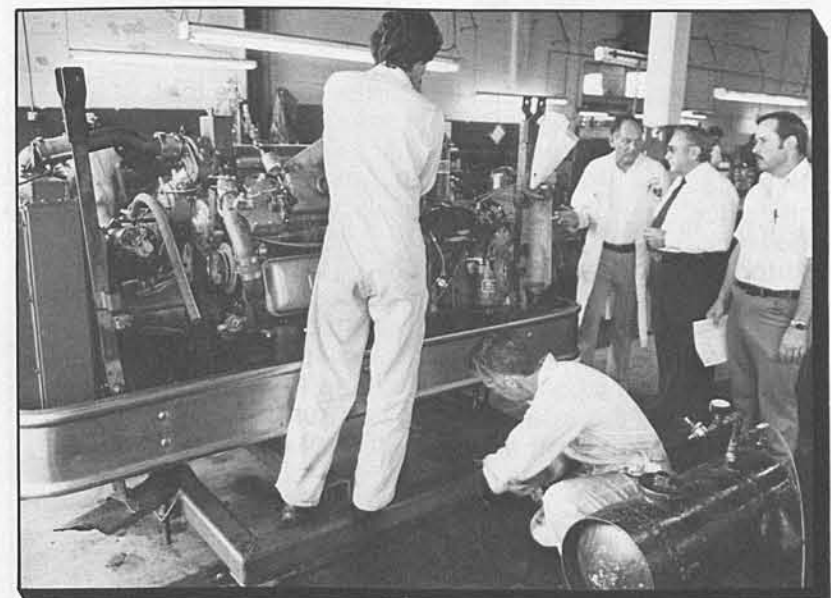
12 At the last station on the line the engine is given a test run prior to installation in a bus. From left are Bill Exline, Jeff Rubin, Charles Dello, L.T. Lenihan, and Howard Sherter.
