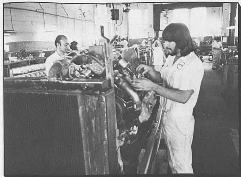
11 As the engine nears the end of the line, Carlos Fuentes (right) and leadman Roy Guzman attach the electrical harness, air shifter and exhaust system.
