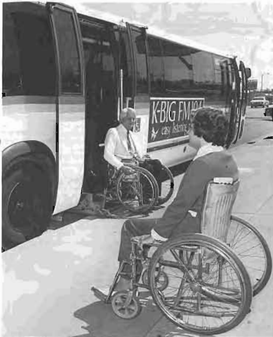
ROLL ON — Expanded accessible service, starting this month, features rear-door lifts on new RTS-IIs.
