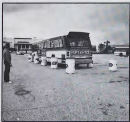
Diminishing clearance requires the operator to maneuver between progressively narrowing rows of barrels.
