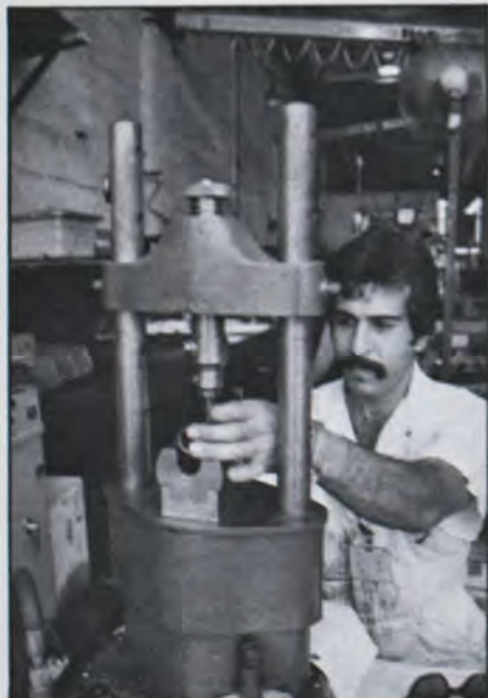
Gary Markarian overhauls cam followers by pressing roller pins into roller bodies.
