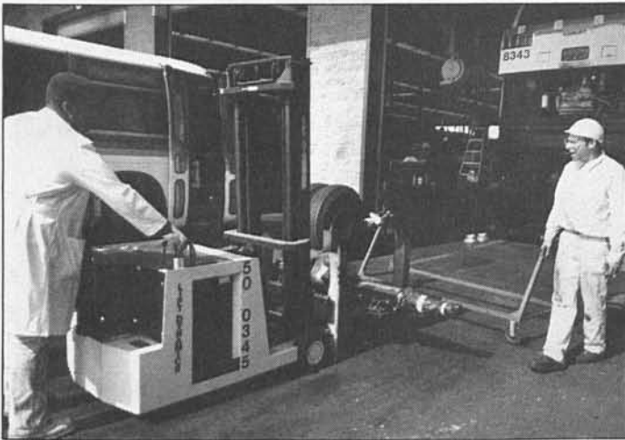
Division 18 Storekeeper Michael McGlothan, left, receives a delivery of a "banjo." A banjo is a mechanical part that supports the differential and is the rear axle of the bus. Mechanic A Steve Grossman, right, had ordered it so that he could complete his repair.
