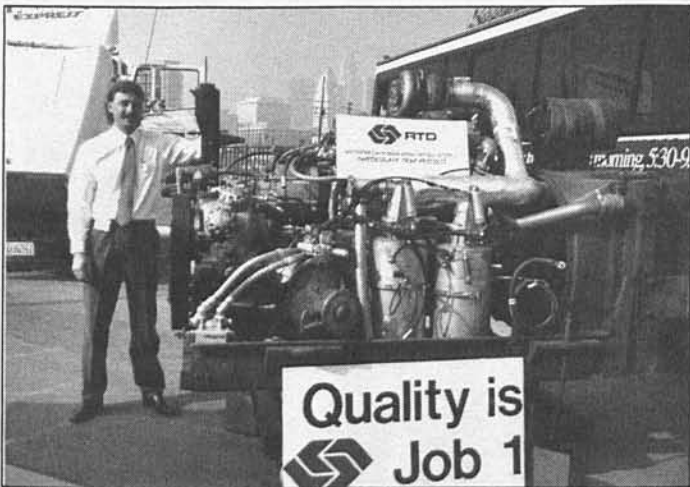
Alternate Fuels Engineer Ray Wilson proudly shows off the RTD's display of a diesel engine with a particulate trap.
