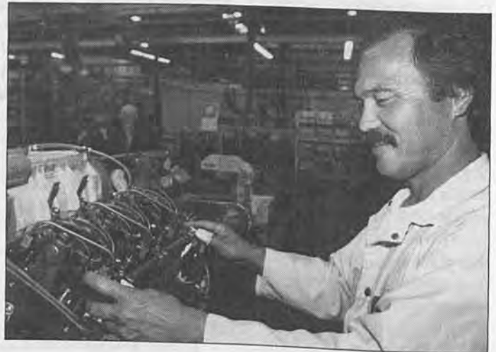
Mechanic A Takata Masamitsu installs an injector fuel rod at Station 5.
