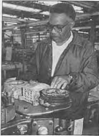
Mechanic A Leadperson Levon Futrell caps the engine with a balance weight cover at Station 2.
