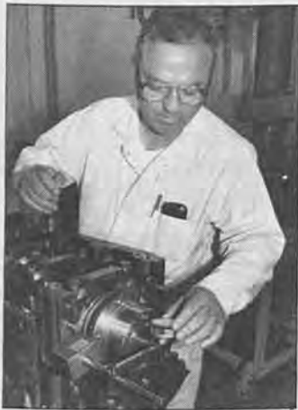
Mechanic A Gene Kenning inspects the crank shaft end play at Station 0.
