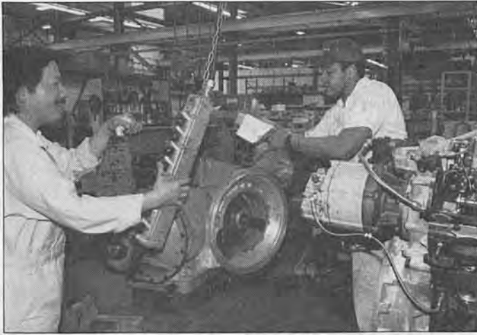
Mechanics A Alfred Chan (left) and Glenn Johnson mount a transmission to the engine assembly at Stations 6 and 7.
