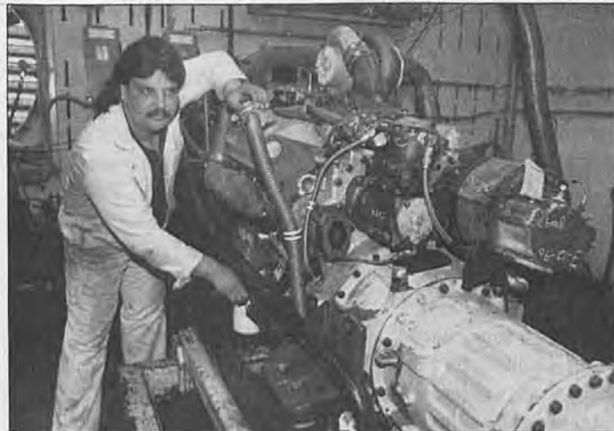
Mechanic A Roman Gonzalez "dynos" the engine and checks for leaks at Station 9
