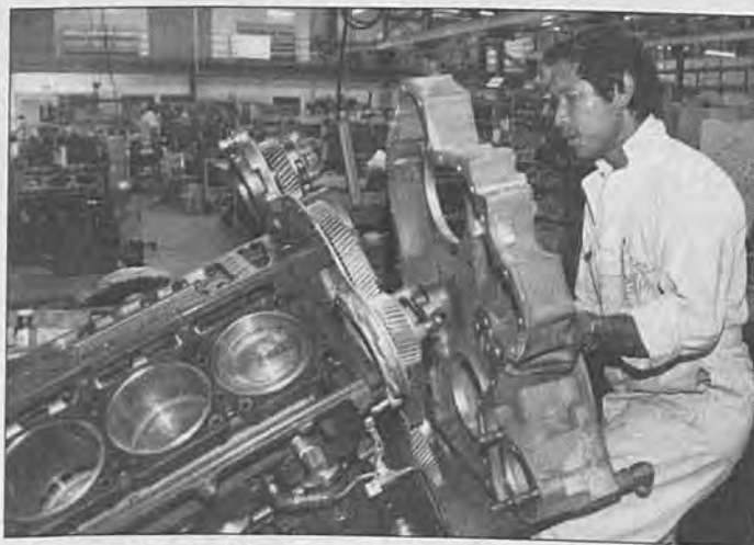
Mechanic A Delphin Wong affixes the engine bell housing at Station 3.
