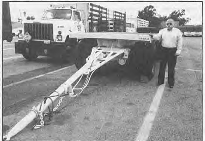
EMS Mike DeGhetto stands beside a 1946 three-axle trailer used by the Los Angeles Transit Lines to maintain the streetcar tracks.
