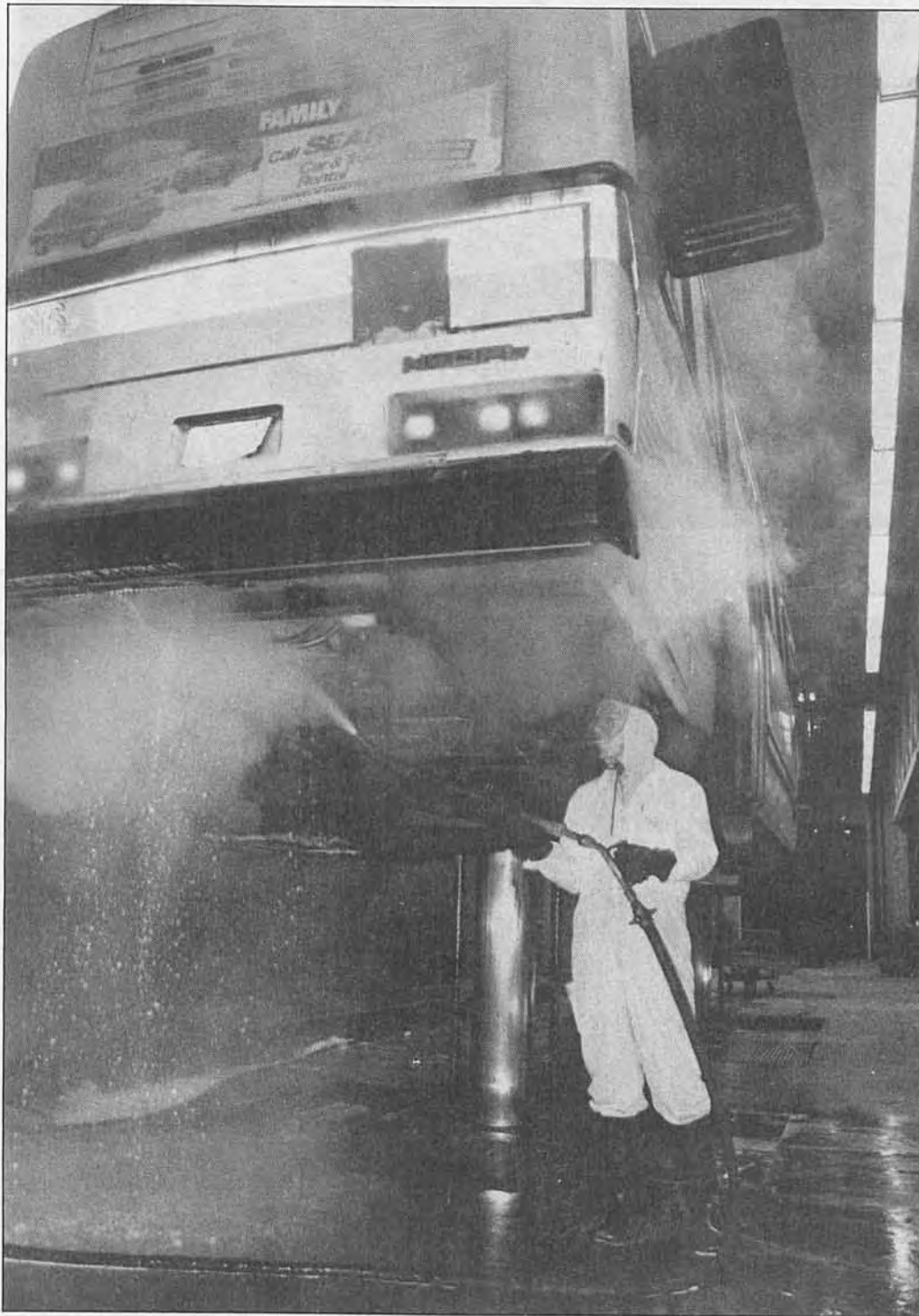
Service Attendant Frank C. Nonn on the night shift steamer. Making the job easier for the mechanics, Frank steam cleans the engines and other parts before repair work on them is attempted.
