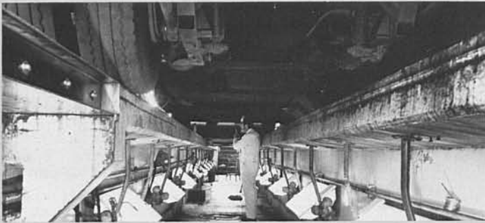
Routine inspection of frame and parts underneath.
