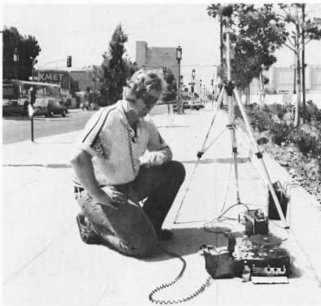
'PULSE READING' — In a sense, one could say that consultant Steve Frost of Wilson, Thrig & Associates is taking a "pulse reading" of Wilshire Boulevard. Actually, the Oakland-based consulting firm was selected by the District Board of Directors to gauge the noise and vibration levels at some 45 points along the Metro Rail alignment. Data will be used in designing the Metro Rail Project to meet environmental standards that will protect the lifestyles of local citizens.
