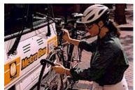
Bike racks already have been installed on the fronts of some 1,400 of the MTA's 2,200 buses. New buses are to be delivered from the factory with the bike racks installed.
