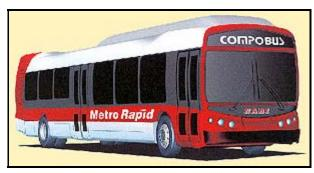
^ The NABI "Compo-Bus" is 45 feet long and seats 47 passengers. Made of lightweight materials, it is CNG-powered.
