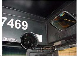
Placed above and to the right of the driver's seat, spot mirrors are positioned so an operator can look up and see passengers boarding. A mechanic can install a mirror in about 15 minutes.
