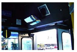
The operators said they used the mirrors to monitor passengers entering the front door of a bus. Analysts had previously concluded that, since the NABI's are low-floor coaches and have no steps, the mirrors weren't needed.
