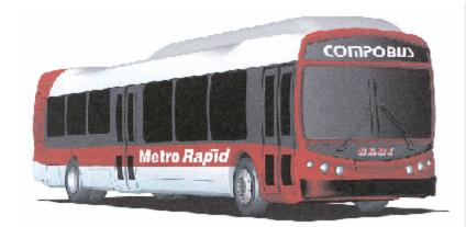
Powered by compressed natural gas, the low-floor "Compo-Bus" will be five feet longer than current MTA coaches and will seat 46 passengers, 16 percent more seats than the traditional 40-foot buses now in operation.
