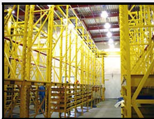
The chemical warehouse provides 4,300 square feet of 15-foot high adjustable storage racks that maximum storage capacity and easy retrieval for hazardous materials.
