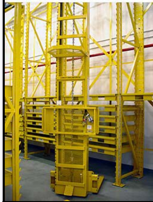
STAK System, which is air motor driven, reduces the need for vehicles in the warehouse.
