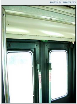
To clean the plastic panel above, Mechanic "A" Leader J.P. Edrich sands it down and then paints over it with a matching color. Below, a rear door access panel before the cleanup process.
