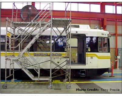
The movable scaffolding shown here alongside a rail car in the Metro Blue Line maintenance shop will be replaced with a safer, more serviceable catwalk.
