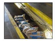
Bags containing 1,000 pounds of sand were used to conduct a weight test on the netting. After two hours, the netting was tested for any deterioration or loss of strength.
