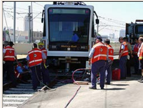
The Metro Gold Line team practices repositioning a train during a derailment exercise.
