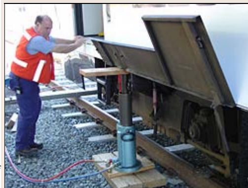
Maintenance Specialist Randy Mittan signals to the operator of the hydraulic jack as the Metro Gold Line train is set back on the tracks.
