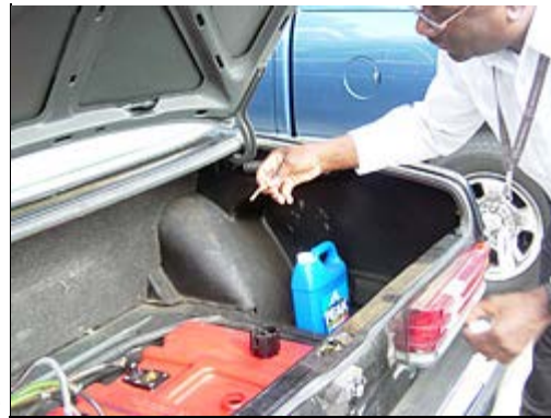
Brown installed a second fuel tank in his trunk to store the vegetable oil. Hoses connect it to the engine.
