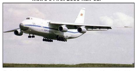
The Russian-built Antonov AN-124 is 226 feet, 9 inches long; 68 feet, 2 inches high; and has a wingspan of 240 feet, 6 inches. The four-engine aircraft has a payload of up to 150 metric tons and can cruise at speeds between 430 and 460 knots for a range of 8,900 nautical miles. The plane's design is similar to the U.S. Air Force Lockheed C-5 Galaxy.
