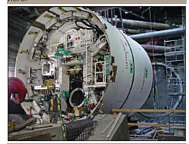
This section will be joined to others to make up the complete earth pressure balance machine.
