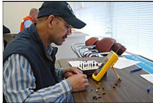
Metro Blue Line Maintenance Specialist Stan Nacon probes for defective components.
