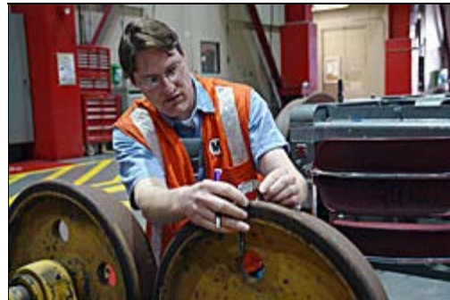
Metro Blue Line Maintenance Specialist Eric Czintos carefully measures the depth and width of the flange on a rail car wheel.
