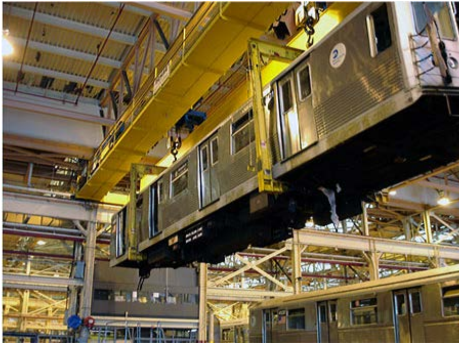
A rail car is hoisted onto a new set of trucks at New York City Transit's maintenance facility.
