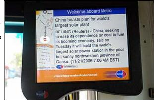
The global positioning map displayed on the left side of the Transit TV screen shows a bus icon located at the real-time position of the Metro bus – in this case, Union Station.
