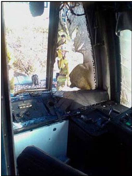
Fire seared the train, causing both exterior and interior damage to the operator's cabin.
