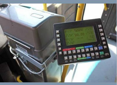
The operator control unit attached to the Cubic GFI Odyssey model Universal Fare System (UFS) fare box allows bus operators to acknowledge receipt of proper fare, classifies the types of passes used or purchased, or note if a rider is short on the fare. Most importantly, it allows riders to use their Transit Access Passes (TAP) to validate their fares.
