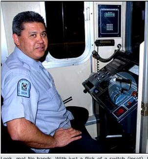
The mode selector knob, inset and below, allows the operator to switch between automatic (ATO) and manual (MTO) modes.
