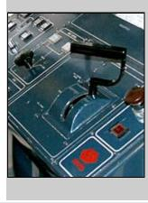
Look, ma! No hands. With just a flick of a switch (inset), Metro Rail Train Operator Robert Rodriguez puts the train in Automatic Train Operations (ATO) mode. But will running in automatic make train operators lose control? No way, says the six-time Rail Rodeo champ. Train operators must make one round-trip in manual mode every shift to keep sharp.
