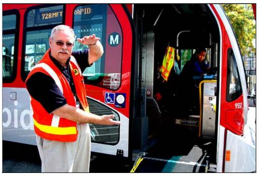
Chip Hazen, Americans with Disabilities Act (ADA) compliance administrator, explains the importance of the wheelchair ramp being deployed at the proper angle, 8.33 percent or lower. He demonstrates that a higher angle could cause a wheelchair to tip over. North Los Angeles Division 3 Bus Operator Quaneka Franklin listens in. *Photo by Ned Racine*
