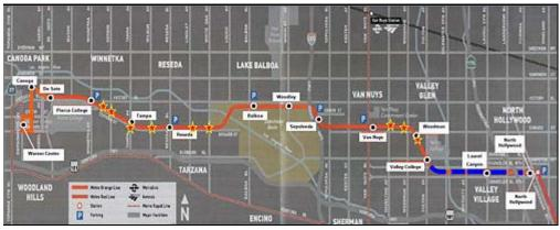
Blue sections represent full-depth pavement replacement; stars mark the intersection approaches where grind and overlay repairs will be undertaken in phase 2.
