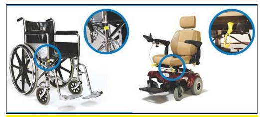
Application of the marking tape and installation of the tether straps, as illustrated above, is done at the request of the patron.
