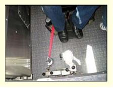
the wheelchair will be secured by linking the bus tie-down to one of the new nylon tether strap that, in turn, would be connected to the wheelchair frame.
