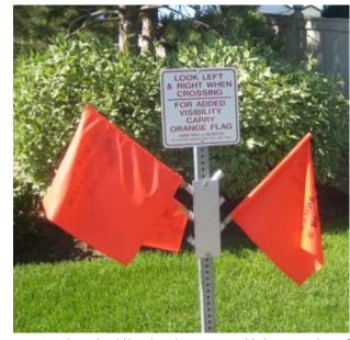
Crossing Flags should be placed in an accessible location, clear of the pedestrian throughway and curb ramps
