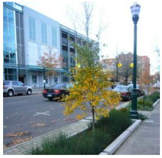
Bioswales manage stormwater runoff, create a natural buffer and beautify the pedestrian environment
