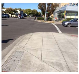
Tighter corners help to manage the speed of turning vehicles
