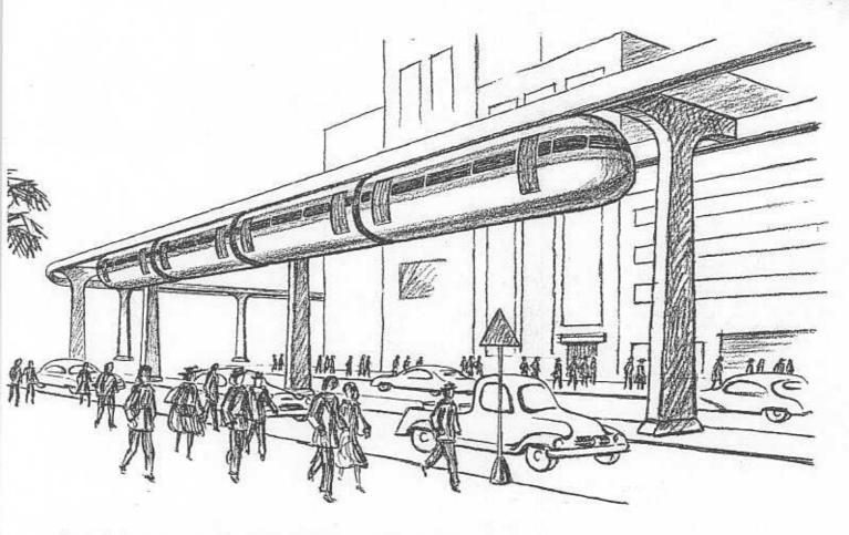
Suspended monorail is sketched above as it might look gliding through Los Angeles. Following a design favored by Gibbs & Hill, the cars are suspended through a slot in the bottom of a girder-like enclosure. The new system, called a "split-rail" monorail, is shown in detail on page 109, along with the "classical," or single-rail, monorail.
