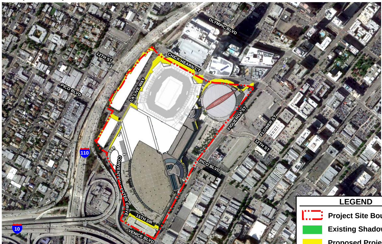
Figure IV.D.1-13 Existing and Proposed Project Shadows During Fall Equinox 1:00pm
