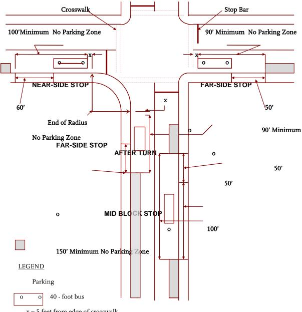
x = 5 feet from edge of crosswalk or end of radius, whichever is further from the intersection.
