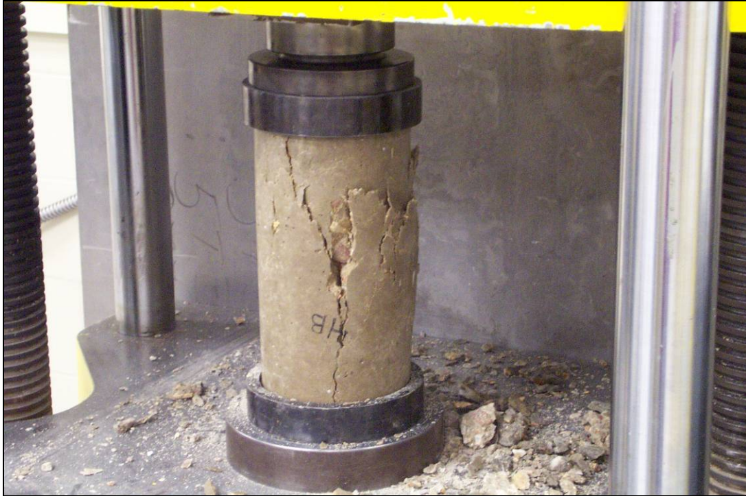
Figure 2: Compressive Strength Testing of Cylinders
