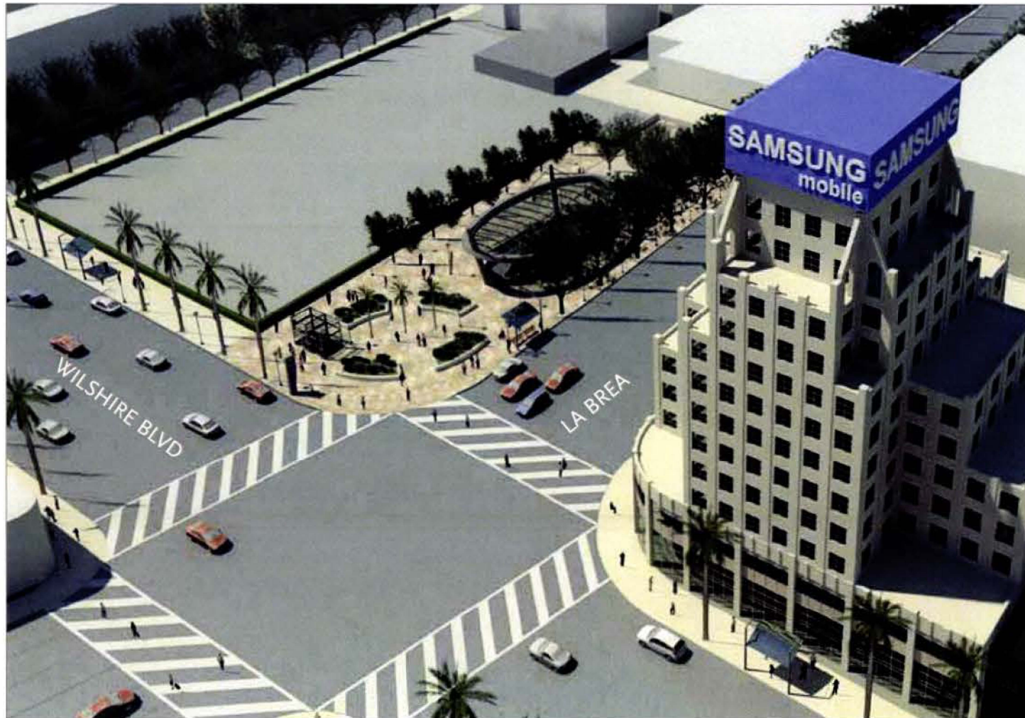
Conceptual rendering (above) explores how the station area will link into the neighborhood, showing the size and scale of the portal, elevators, circulation pathways and landscaping.
