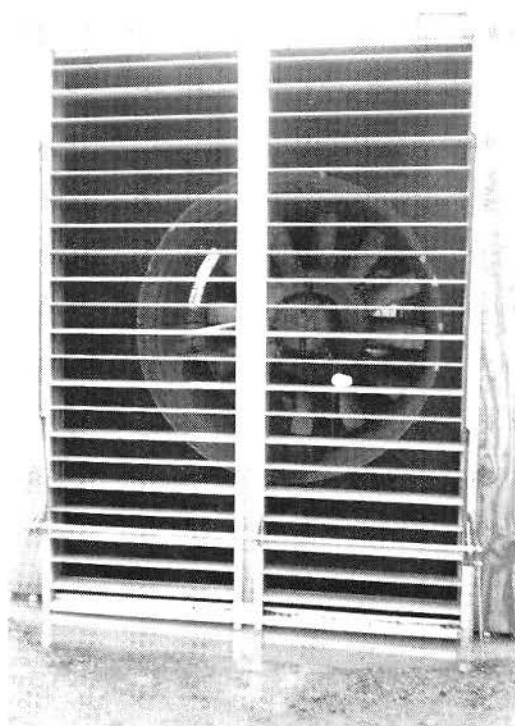
SUBWAY VENT FAN & DAMPER BEING TESTED FOR TRANSIENT PRESSURE CHARACTERISTICS
