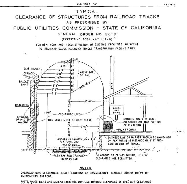
OF 10-0" IS RECOMMENDED WHERE PRACTICABLE. ALL SIDE CLEARANCE DIMENSIONS ARE FOR TANGENT TRACK. IN GENERAL SIDE CLEARANCE FOR
